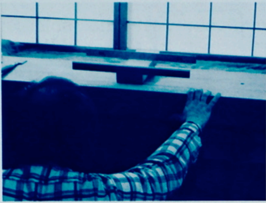
Left: Using the winding sticks to sight for winding in the plane body. Below: The configuration of the sole can be seen by placing a straight edge along the length of the body and observing the light.
